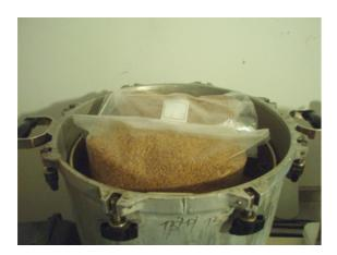
Get the lid locked and put the cooker on a hotplate and start the heating. Wait until you can see steam leaking
