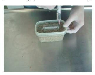
Should the needle touch anything unsterile, you will have to sterilise it again. Therefore hold the nip of the needle into a flame (Bunsen burner or lighter) until the nip turns red and let it cool down again. (Do not overheat the needle as the stand is made of plastic which could melt!)
